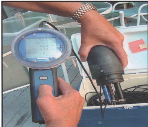
Figure 2. Hydro-Lab with receiving apparatus
