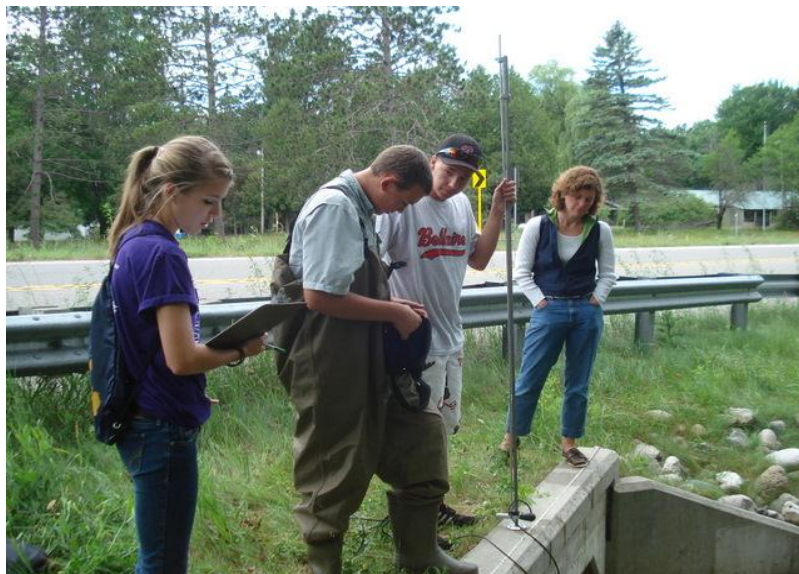
Figure 1. Determining the cross-sectional area of Shanty Creek
