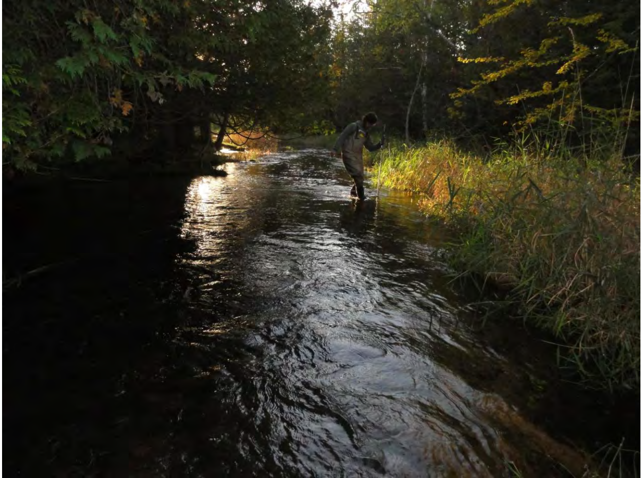
Figure 4. Blaze Budd measuring discharge using the wading method (with the OTT ADCM) along the upper Rapid River near sunset.
