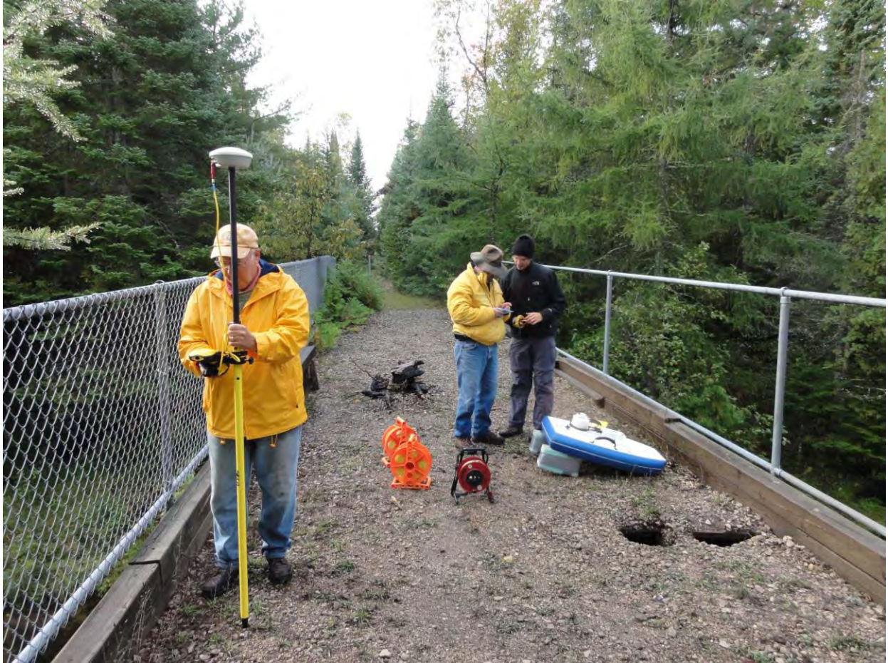
Figure 1. Bob Kingon of the Elk-Skegemog Lake Association collecting a GPS measurement on the Cut River. In the background, Lon Cooper (in yellow) and Anthony Kendall (in black) prepare for a stream discharge measurement using the ADCP (white and blue boat).
