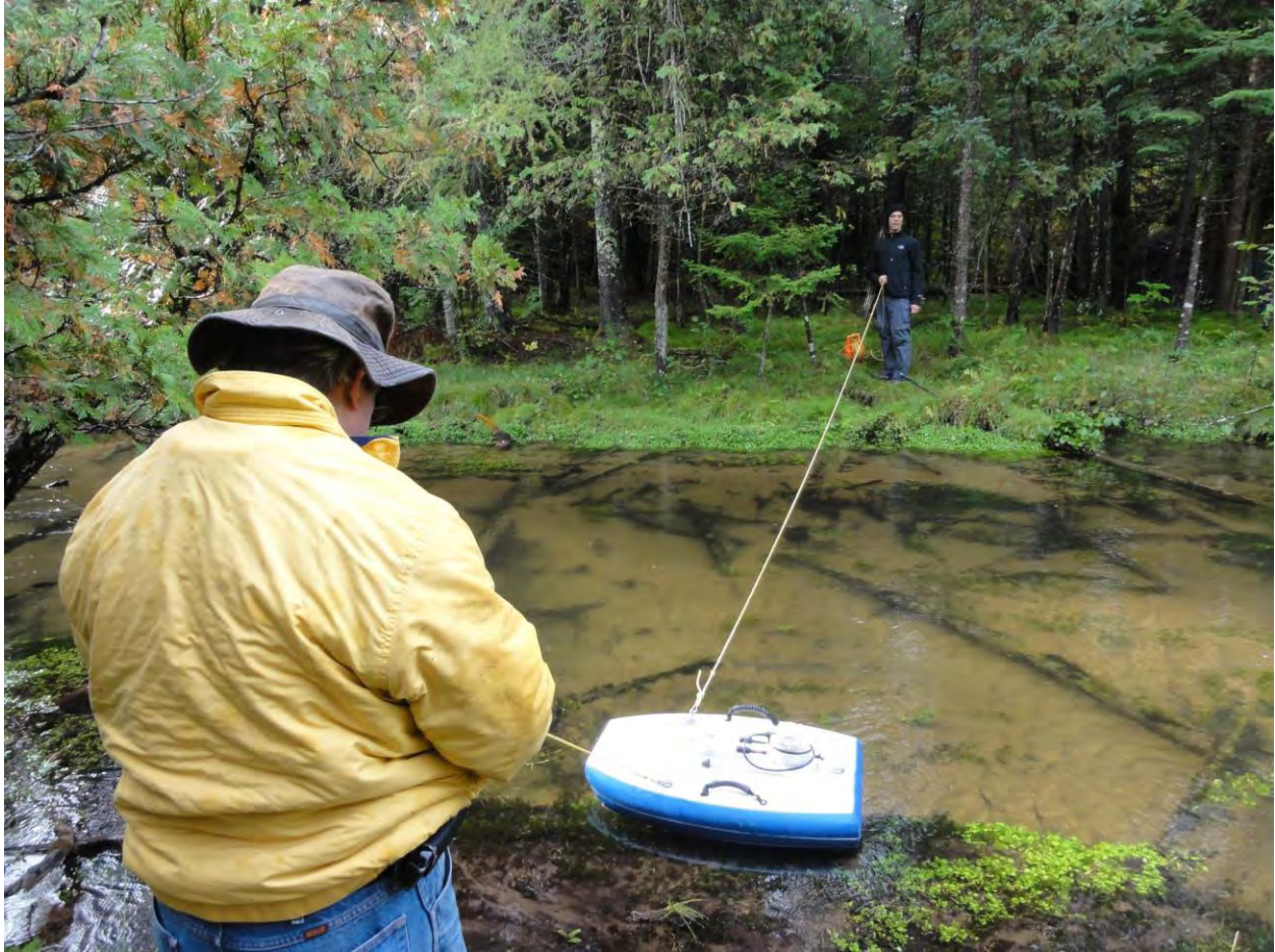
Figure 2. Lon Cooper and Anthony Kendall pulling the ADCP across Shanty Creek, a tributary of the Grass River, the measure stream discharge and channel geometry.
