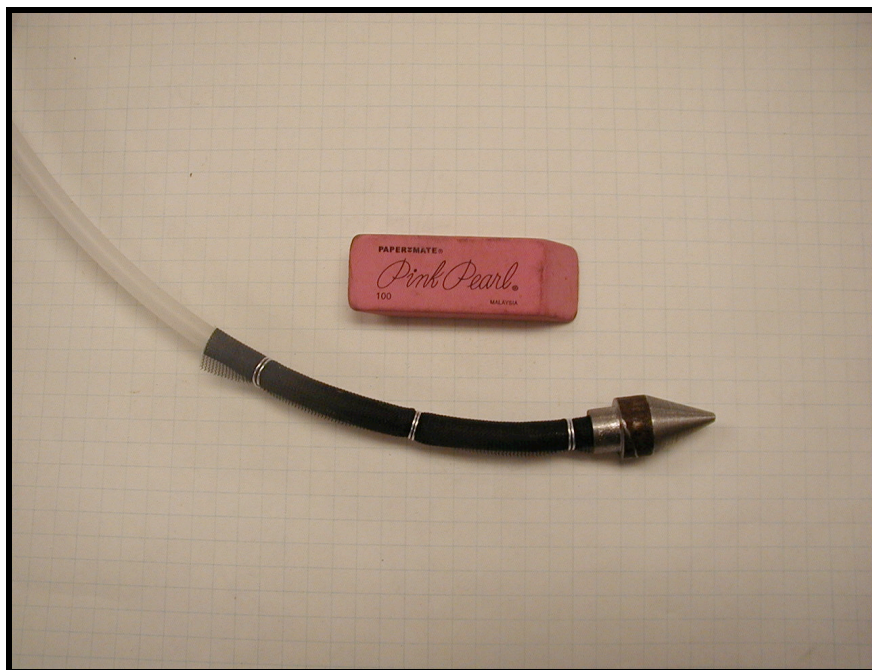
Fig. 7 - Well point, mesh screen, and sampling tube
