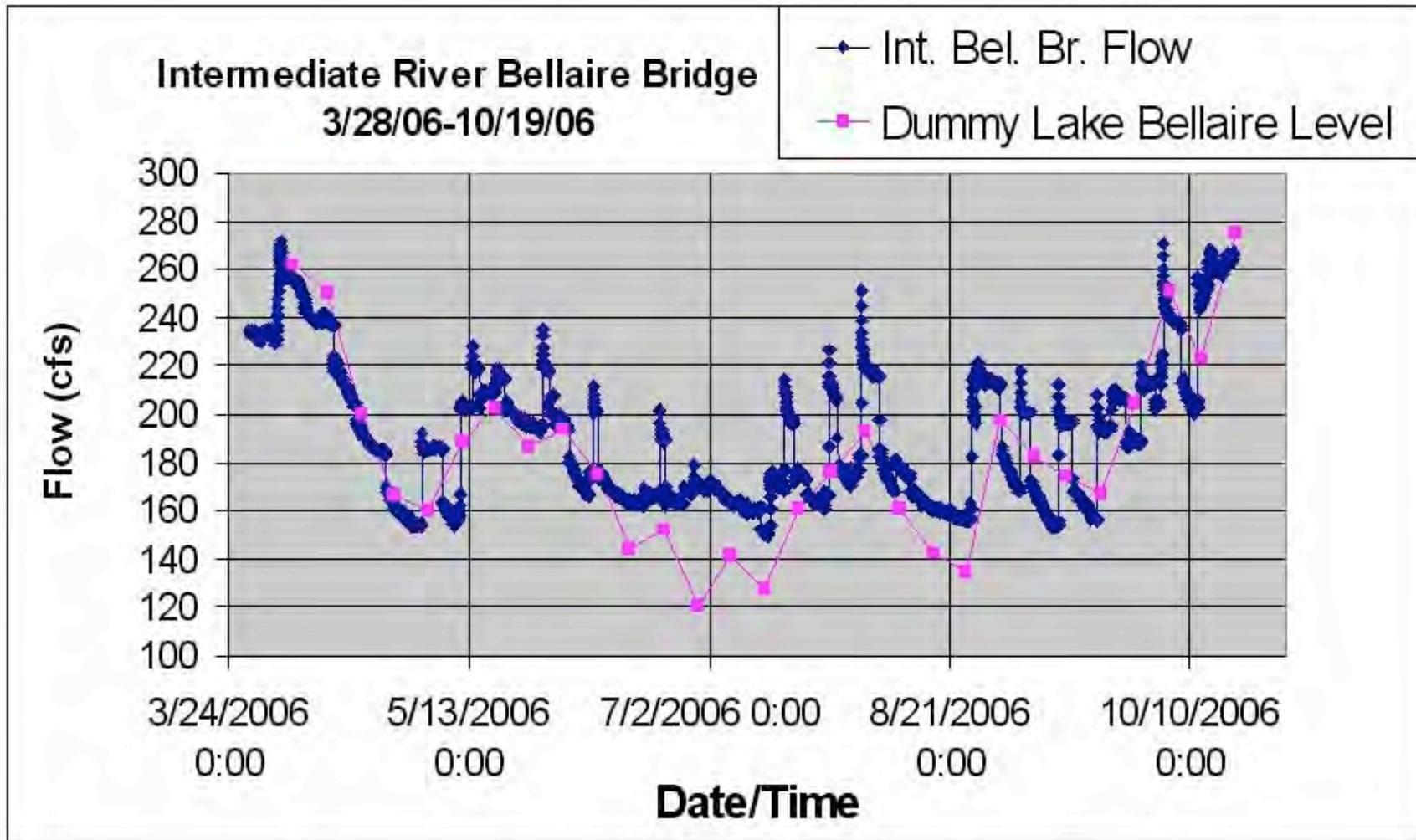
Fig. 7c Flow data on Intermediate River below the Bellaire Dam taken at hourly intervals. Abrupt jumps in flow correspond to openings and closings of the dam to keep the level of Intermediate Lake approximately constant. Also shown is value proportional to the Lake Bellaire Level.
