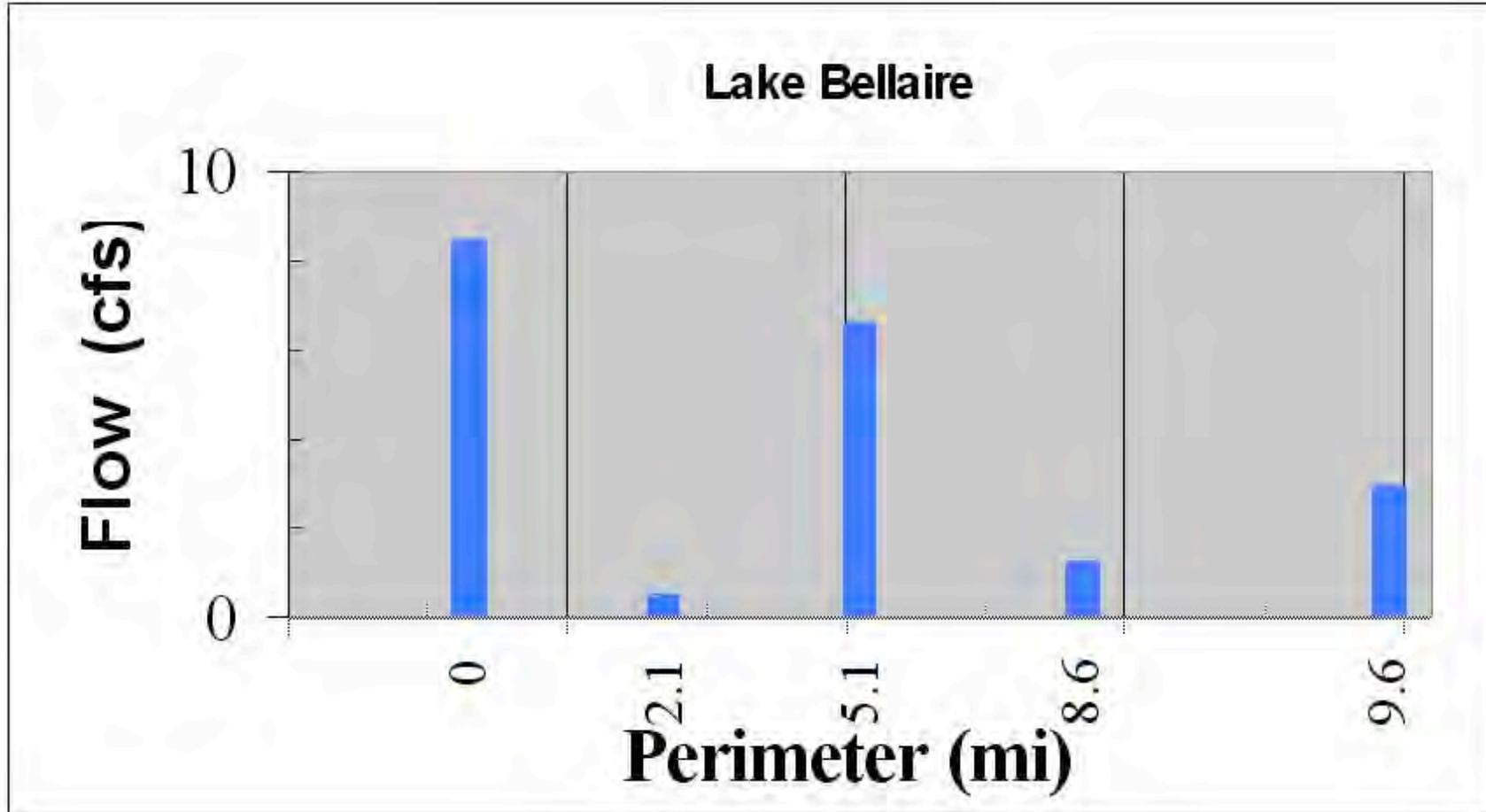
Groundwater flow (cfs) versus Lake Bellaire perimeter clockwise starting with north central piezometer station #1.
