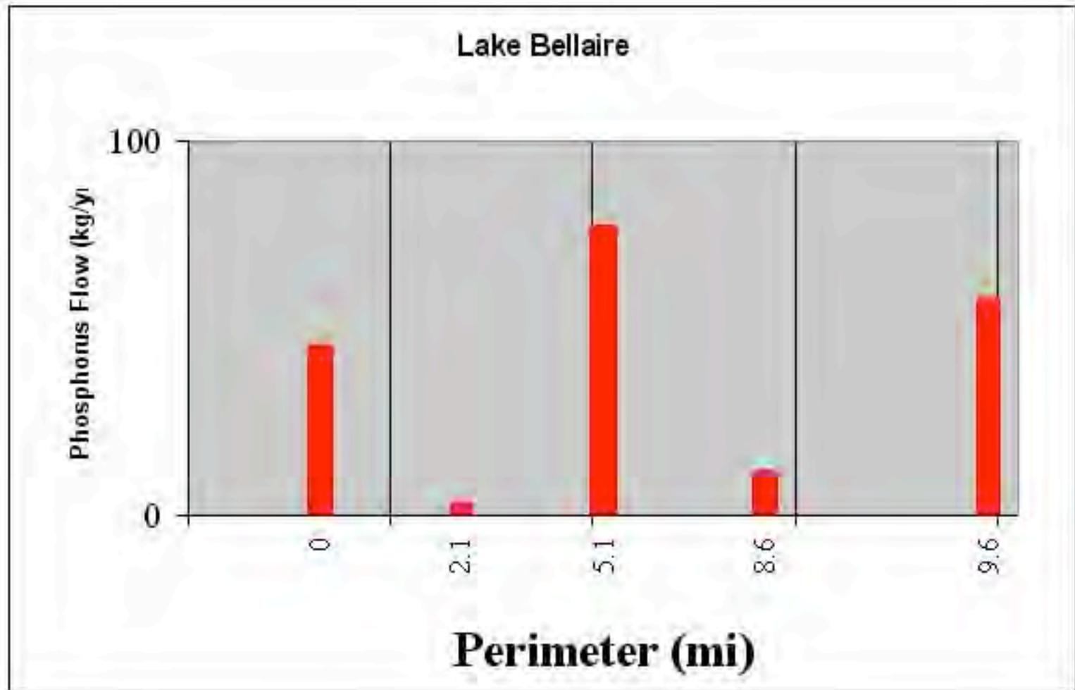
Groundwater phosphorus flow (kg/yr) versus Lake Bellaire perimeter clockwise starting with north central piezometer station #1.
