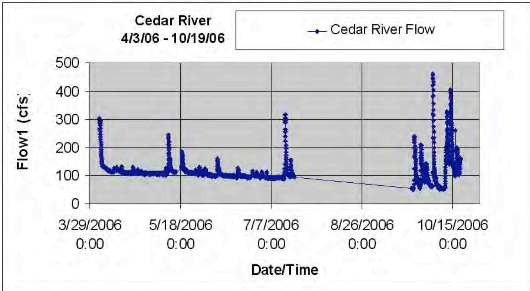
Fig. 7a Flow data from an automated gauge on the Cedar River taken at hourly intervals. The gap in the flow was caused by a gauge failure.
