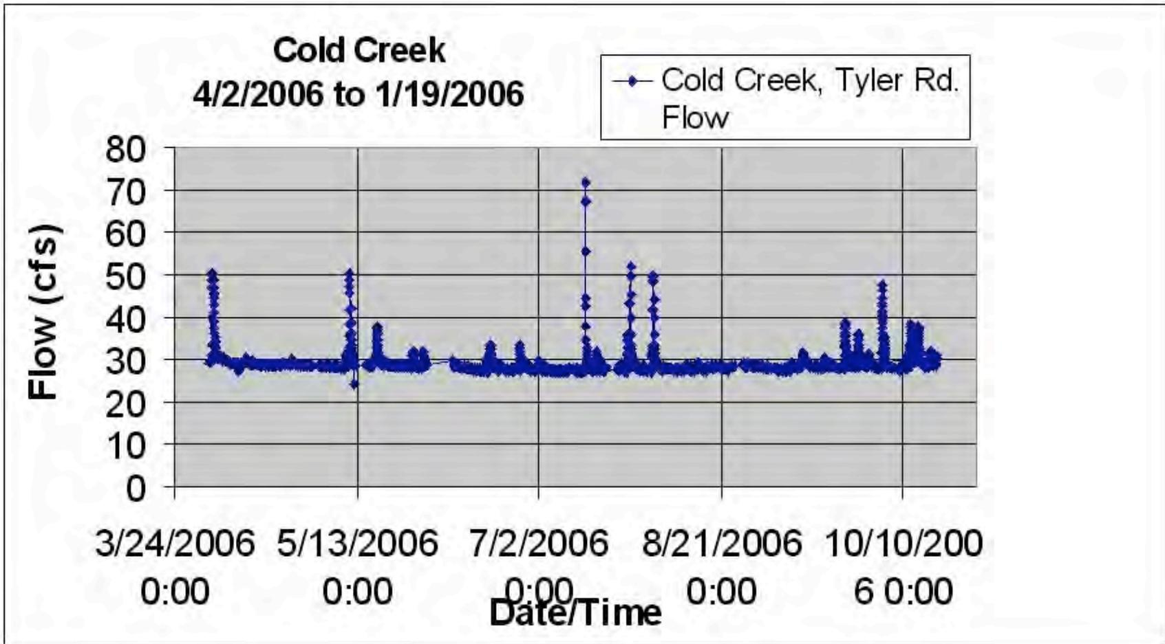
Fig. 7b Flow data on Cold Creek from an automated gauge at hourly intervals.
