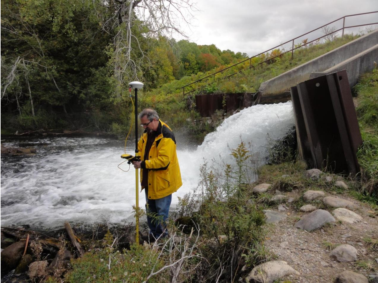
Figure 10. Lon Cooper collecting a GPS elevation measurement below the secondary spillway of Rugg Dam.
