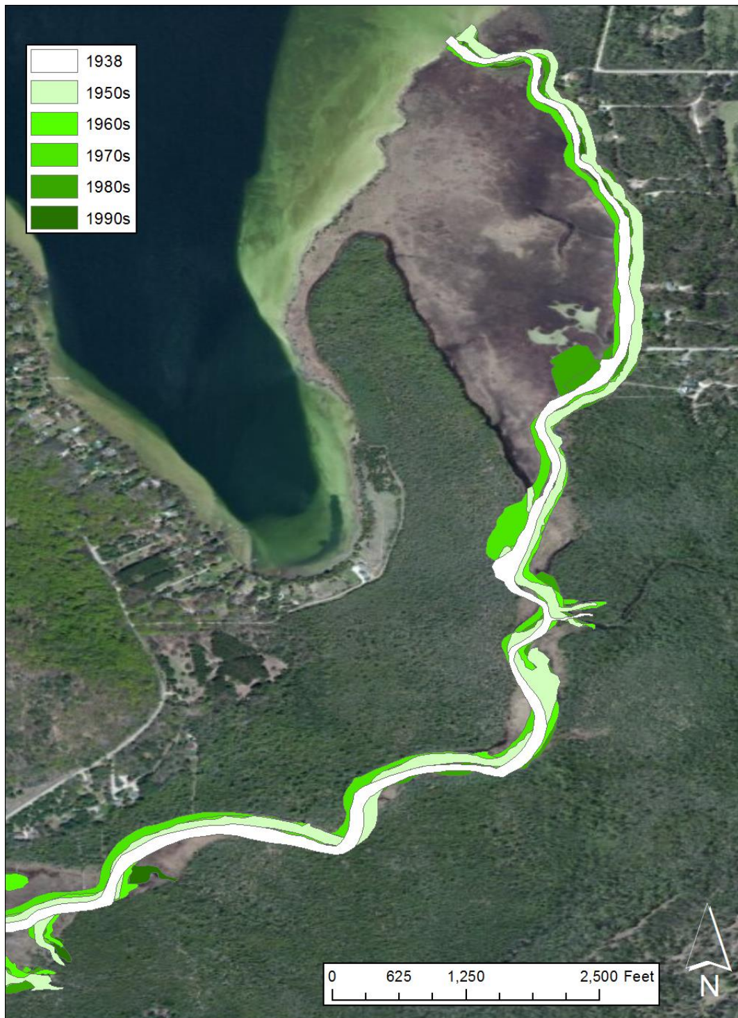
Figure 29. Map of the Grass River through time as digitized from historical aerial imagery. Note that the positions of the streams are not as accurate as the geometry. Thus the shifts in the channel should not be interpreted as genuine, but the shape of the channel and its dimensions are accurate.
