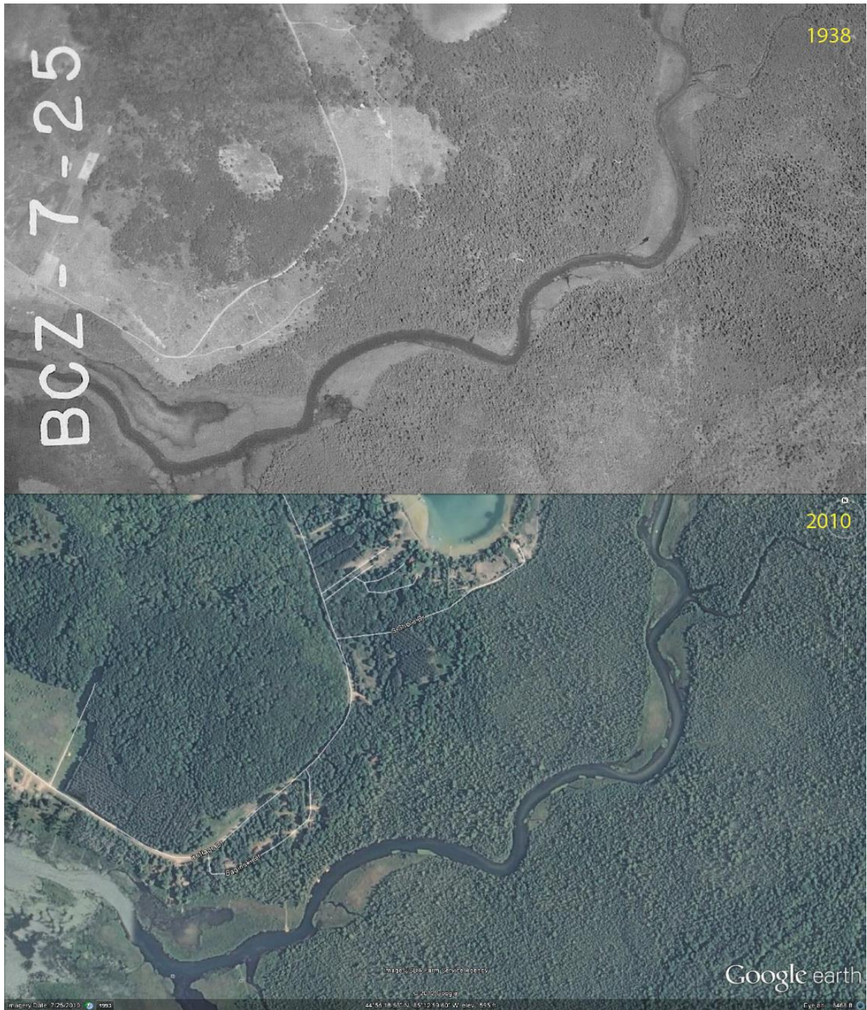
Figure 28. Comparison of the same frame (Grass River at the mouth into Clam Lake) between 1938 and 2010. The 2010 channel is significantly wider, and new mid-channel sediment features have developed downstream of Cold Creek.
