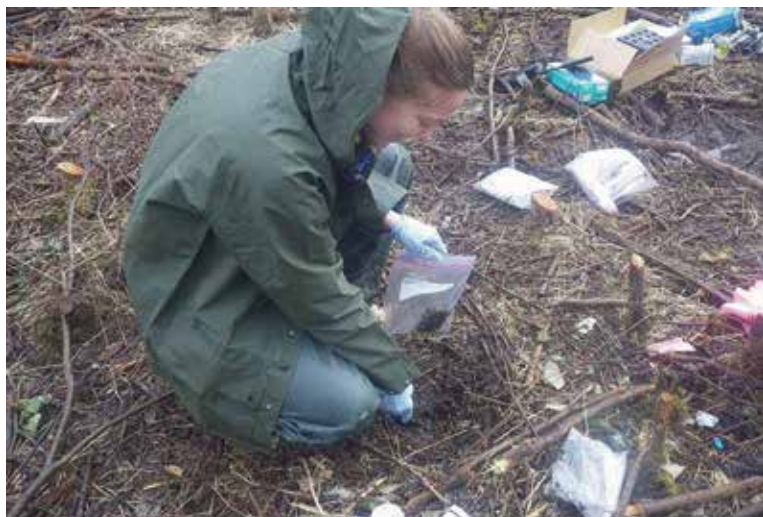
Samantha Fox collecting a soil sample from a contaminated site in Alaska to be analyzed for the amount of spilled petrochemical hydrocarbons in the sample.
