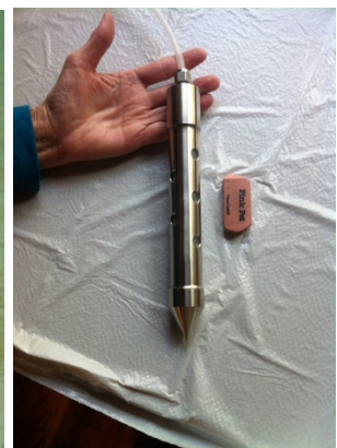
Temporary piezometer point
