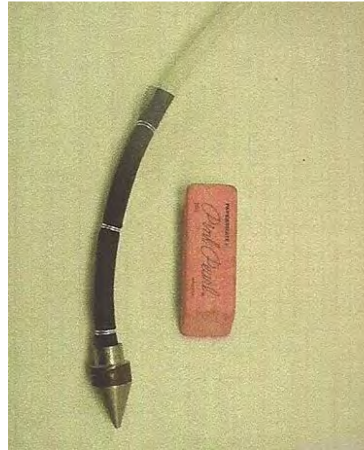
Small Piezometer Point and Screen
