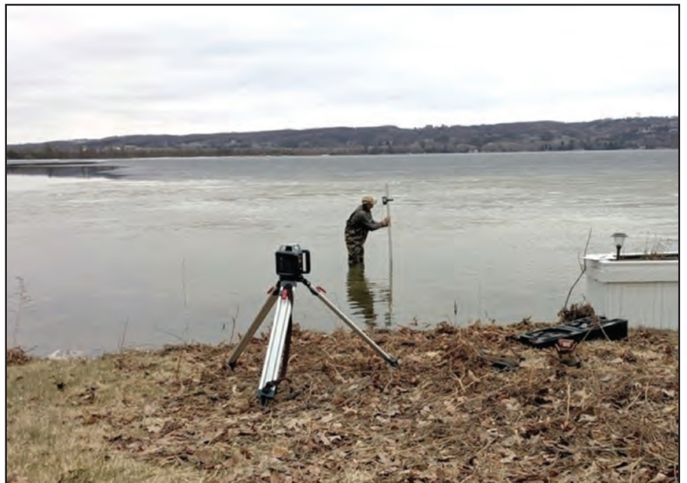
Setting up a lake level measuring location on Lake Bellaire
