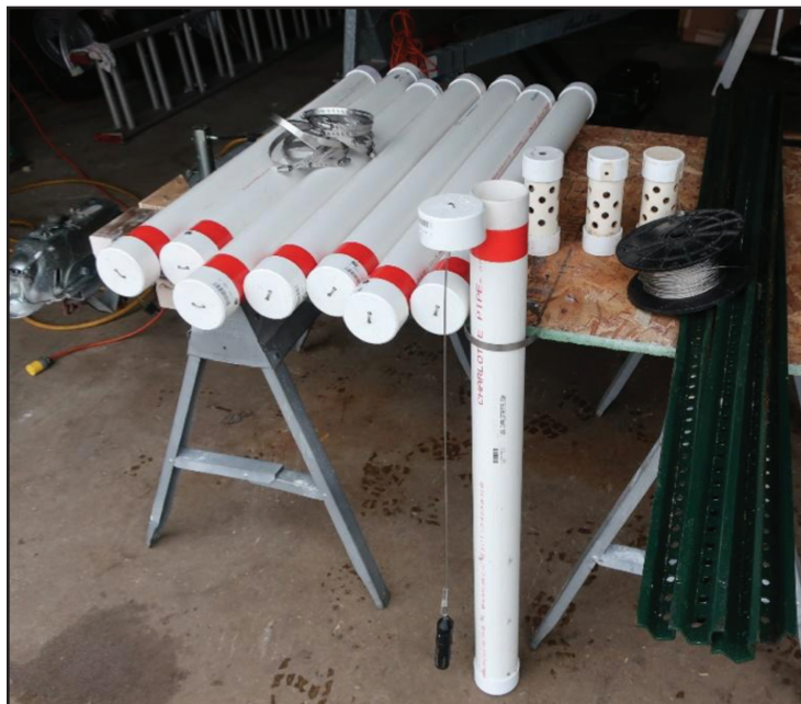
Stilling wells fabricated from three-inch diameter sections of PVC drain tube. The well standing vertically in the foreground has the top cap removed revealing the level logger (black) hanging from its support cable.
