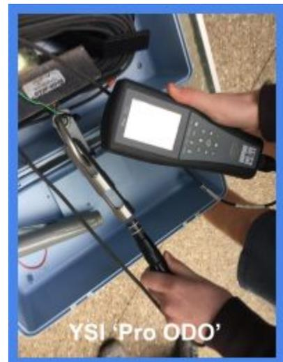
Note that for both the July and August measurement sessions, the Hydrolab 'Quanta' and the YSI 'Pro ODO' were not properly calibrated for collecting dissolved oxygen data due to a lack of available materials and technical difficulties. However, this does not affect the temperature data and those available readings should be accurate.
