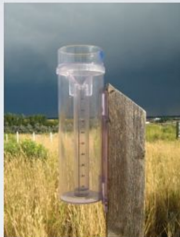
4-inch diameter high capacity rain gauges
